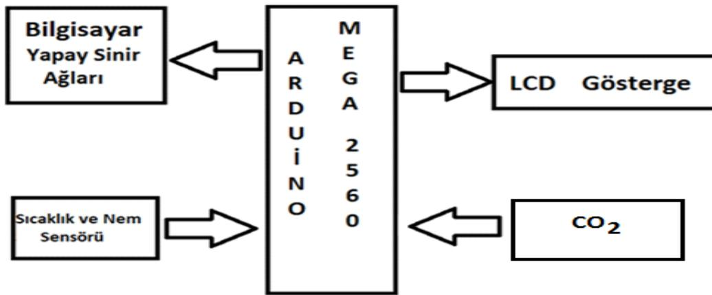
**Figure 3.** Block Image of Measuring Assembly
