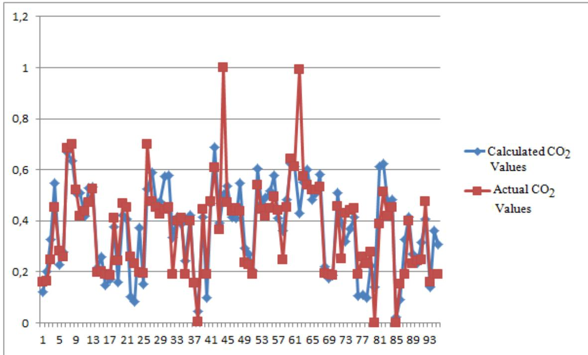
**Figure 10.** Comparison of Indoor Sports Hall's actual and calculated CO<sub>2</sub> values
